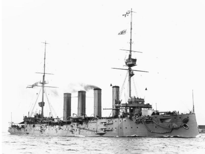
H.M.S.GOOD-HOPE, cruiser with 2 x 9.2" and 16 x 6" guns, flagship of Rear-Admiral Cradock
